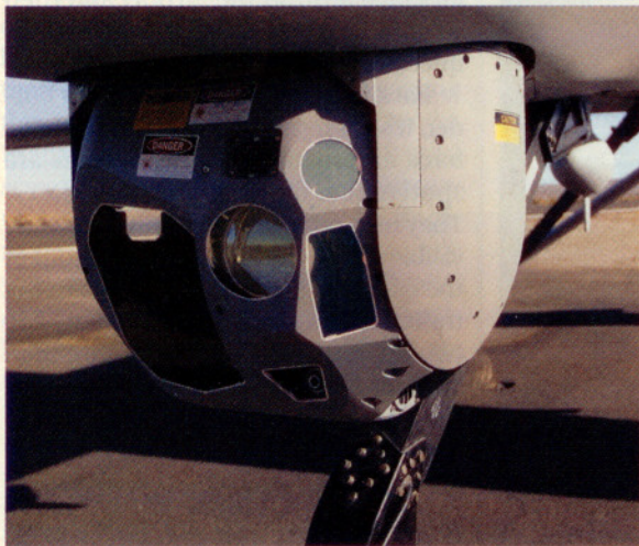
A microwave communication link with Predator A at El Mirage (far left). Predator A awaits a training mission at General Atomics' El Mirage facility (above). The payload is a gimbals-mounted camera that can include a wide array of potential instruments including high-resolution visible and infrared cameras as well as muzzle-flash detectors and laser-imaging devices (left).
